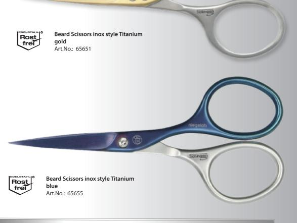
Valuable stainless steel and titanium nitride alloy of one half of the scissors produce the self-sharpening effect. The hardening of the cutting bit achieved by the titanium nitride alloy, which is now about twice as hard as the uncoated cutting ridge of the scissors, causes the harder and more wear-resistant cutting edge to re-establish the softer one at each opening and closing. Thus, the scissors retain their cutting sharpness much longer as other scissors.
